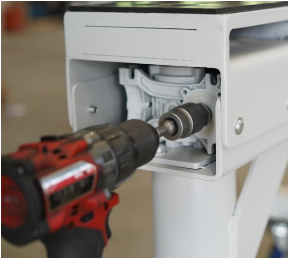
Cordless screwdriver drive via gearbox connection
